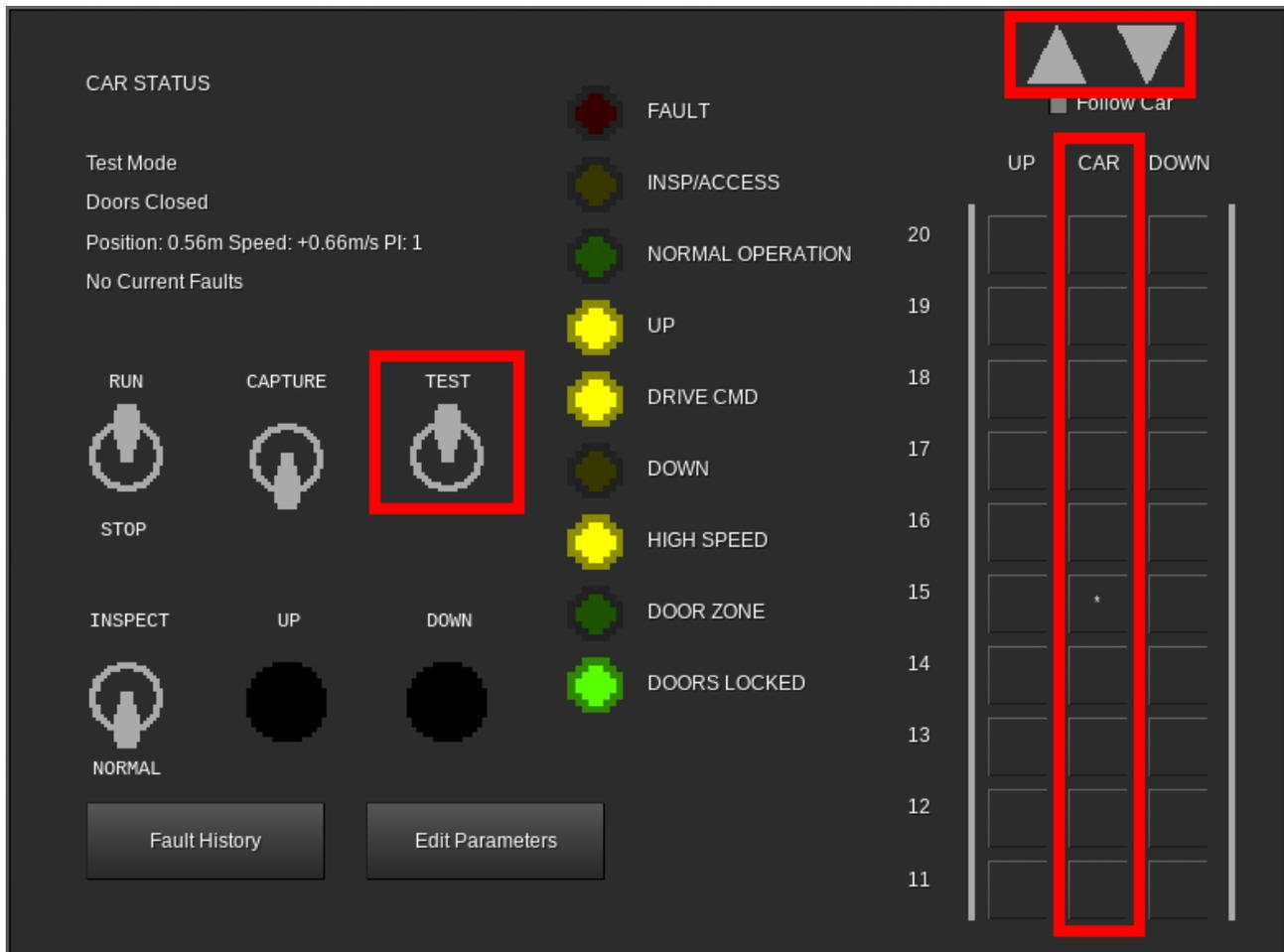
One at a time, click each floor in the **CAR** column. This will place a car call (indicated by an asterisk) on that floor. After placing each call, observe the car and verify that it stops properly at the floor, then continue on to the next floor. Due to test mode being enabled, the doors will not open when the car stops.
